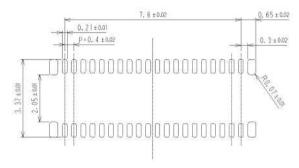
Recommended soldering paste amount: 0.0121 mm<sup>3</sup> (Per 1 Pad)
