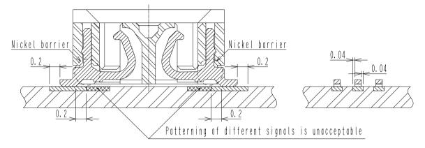
Pad layout and connector position for plug
