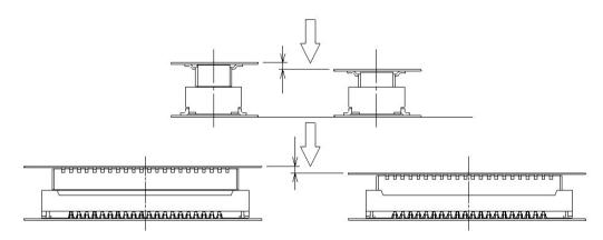
3) Once aligned, the connector pair does not move back and forth and around as they are located in a parallel position. Mate the connectors completely by applying force in this condition. We recommend to push the connector with two fingers for 50 pins or more to press down the whole connector evenly. One end might not be inserted enough to result in half mating for high pin counts.
