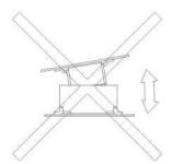
3) Check the rigidity of the FPC for unmating operation prior to your production, otherwise solder breakage and/or connector breakage may occur during unmating process. Lift up the corner of the FPC could apply over stress to the contacts.
