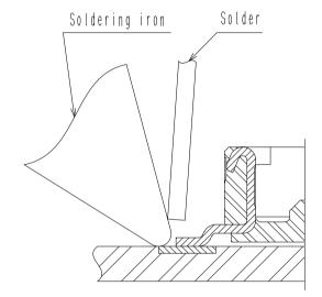
It may affect on mating that the soldering paste height is 0.17 mm of more from the upper surface of the plug contact.
