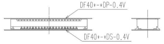
4) Make sure that the connectors are mated completely. When the PWBs are not parallel, unmate the connector, and then mate them again according to the above procedures from the beginning.
