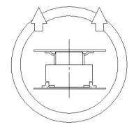
2) When vertical removal is difficult, lift up either side of longitudinal, contact pitch direction. Do not unmate the connector in connector width direction otherwise the contacts could receive great stress.
