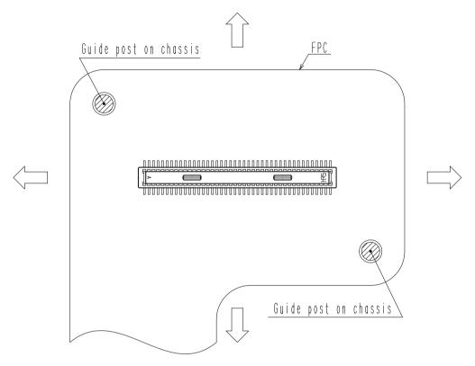
EX) Inflexible FPC positioning with guide posts on chassis as shown above disturbs flexibility to the directions indicated by arrows.
