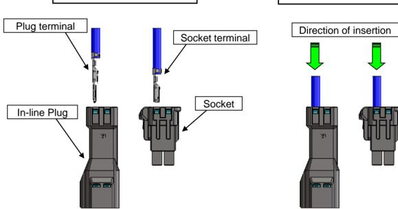
• For insertion, place the crimped terminal and crimping socket lock in the following direction:
