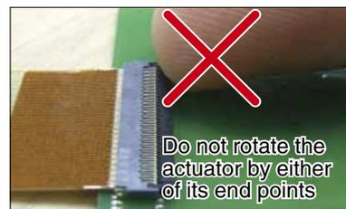
This connector uses a back flip type structure. The direction of the FPC insertion and that of the actuator are different from front flip type connectors. Do not try to open the actuator from the FPC side.
