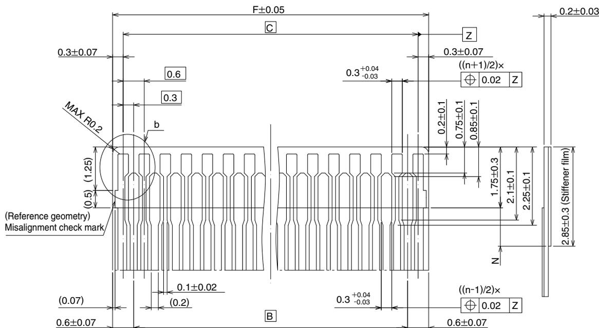
Note 6: FPC should be designed so that the dimension of N is 0.5 mm or more.
