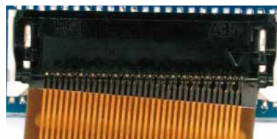
FPC is inserted diagonally.
