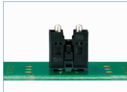
③ Interposer Installed
