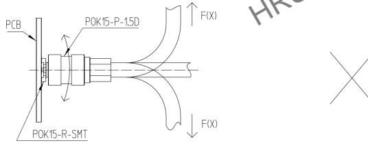
\* If you use this product without the fixing structure, If the force acts in the direction differently from the center of the product, it may cause the loss of function due to eccentricity of the product.
