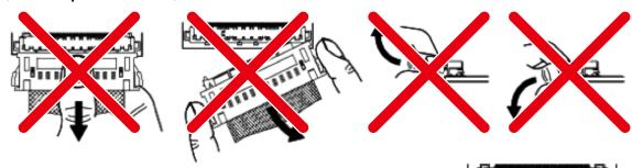
[3] In the case when the connector has been unmated forcibly.
