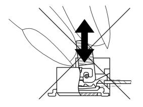
•Release the actuator to remove the FPC.
