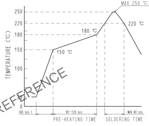
Reflow method: IR reflow Number of reflow cycles: 2 cycles MAX. Duration above 220°C, 60 sec MAX. (Peak temperature:250℃ MAX) Pre-heat temperature(MIN):150℃ Pre-heat temperature(MAX):180°C
