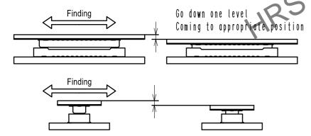
(2) When quiding, the connectors are aligned parallel to each other, with longitudinal and lateral movements restricted. Mate them properly by applying force in this condition.
