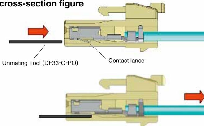
1. Insert the unmating tool and move or disengage the contact lance. (as shown in the example on the left)
