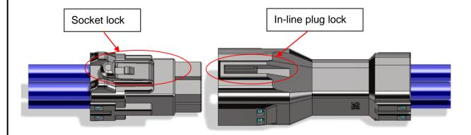
Fig.2 Positioning for insertion
