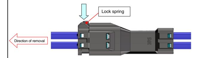
Fig.6 Socket removal
