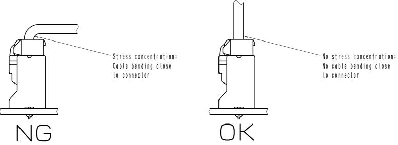
2) When applying load to connector end, please use the retainer for reducing the stress affection on the connector. Retainer shall be installed after inserted crimping contact completely. It might be impossible to insert it when terminal installation is incompleted.
