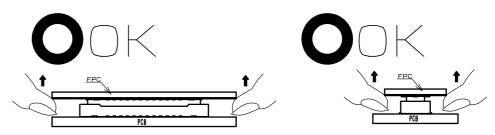
(≥) IF THE CONNECTOR CANNOT BE UN-MATED PARALLEL IT CAN BE REMOVED DIAGONALLY FROM THE PITCH DIRECTION. TO DO SO SINCE THIS ACTION APPLIES STRESS ON THE CONTACT.
