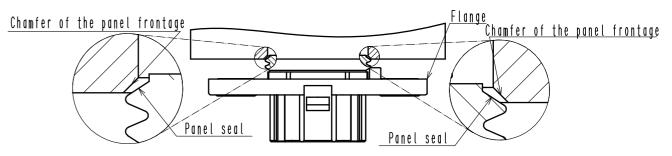
While in this position, press on the male connector housing or collar and push the male connector straight into the enclosure opening. Push straight in until the male connector flange touches the panel.
