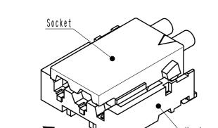
②Slightly press the socket down at cable side to tilted angle.
