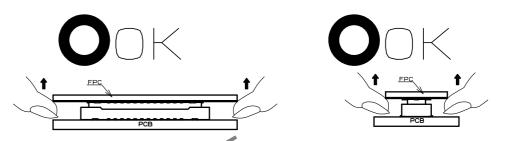
(2) IF THE CONNECTOR CANNOT BE UN-MATED PARALLEL IT CAN BE REMOVED DIAGONALLY FROM THE PITCH DIRECTION. DO SO SINCE THIS ACTION APPLIES STRESS ON THE CONTACT.
