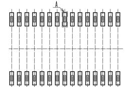
Connector lead on PAD layout
