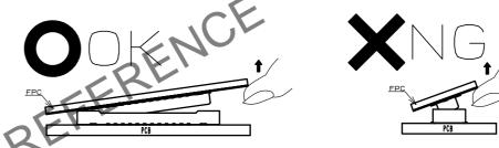
(3) IF THE FPC IS NOT RIGID, THE CONNECTOR CAN BE BROKEN. PLEASE CHECK THE ACTION OF THE FPC TO BE USED REPEATEDLY AT THE TIME OF TRIAL PRODUCTION. BE CAREFUL TO UN-MATE THEM FROM THE PITCH DIRECTION, PULLING IT FROM THE CORNER CAN ALSO RISK TO PUTTING STRESS ON CONTACTS.
