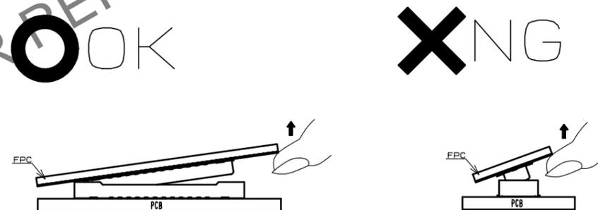
(3) IF THE FPC IS NOT RIGID, THE CONNECTOR CAN BE BROKEN. PLEASE CHECK THE ACTION OF THE FPC TO BE USED REPEATEDLY AT THE TIME OF TRIAL PRODUCTION. BE CAREFUL TO UN-MATE THEM FROM THE PITCH DIRECTION. PULLING IT FROM THE CORNER CAN ALSO RISK TO PUTTING STRESS ON CONTACTS.
