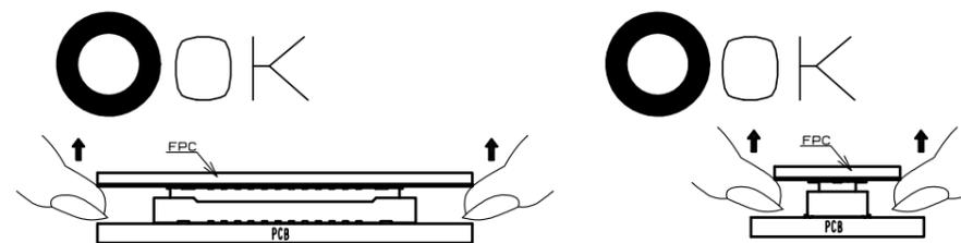
(2) IF THE CONNECTOR CANNOT BE UN-MATED PARALLEL IT CAN BE REMOVED DIAGONALLY FROM THE PITCH DIRECTION. BE CAREFUL TO DO SO SINCE THIS ACTION APPLIES STRESS ON THE CONTACT.
