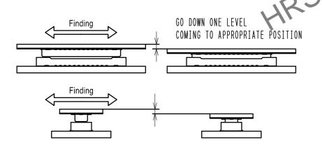
(2) WHEN GUIDING, THE CONNECTORS ARE ALIGNED PARALLEL TO EACH OTHER, WITH LONGITUDINAL AND LATERAL MOVEMENTS RESTRICTED. MATE THEM PROPERLY BY APPLYING FORCE IN THIS CONDITION.
